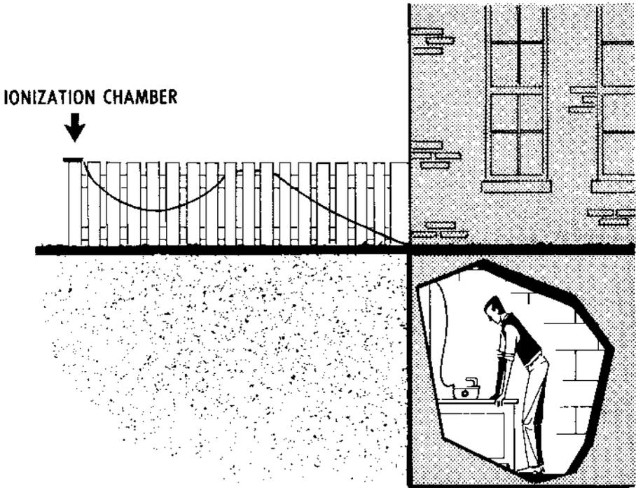
ILLUSTRATION 4.4—Taking reading with the CD V 717.
